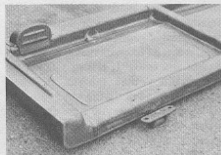
TOP LEFT AND RIGHT, before! This sidegate from a VW pickup shows the accumulation of several years rust. ABOVE, after! The sidegate looks as good as new after being stripped clean and sprayed with a protective coating.
