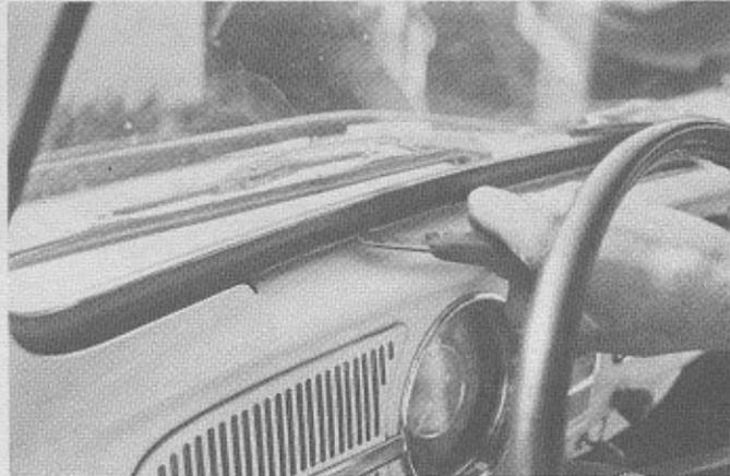
**ABOVE**, the preceding six steps show how the two side windows are replaced in a Bug. The rear window is done in the same manner, though it is a little more difficult because of being bigger. The front windshield, however, has to be treated much more carefully as it is weaker. To begin with, the old rubber gasket has to be cut away with a knife so that the windshield can be lifted out without force. Replacing it is done in much the same way, but far more carefully.
