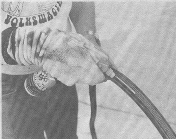
**STEP 2**, liberally coat the new rubber with Armor All, or a similar rubber lubricant. This helps keep the rubber alive longer as well as making the installation easier.
