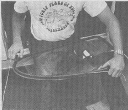
**STEP 4**, slip a long piece of strong, thin string around the window rubber, in the groove that will hold the glass in the window frame.
