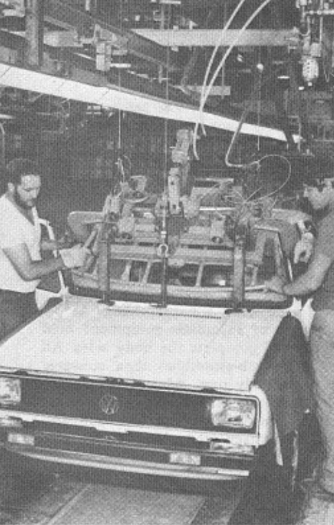
LEFT , the windshields arrive on an overhead conveyor. Perfect body jigs are needed to assure correct fit. BELOW , assembly line has stands for mounting each body on a "spit" for ease of welding and assembly. CENTER , a look inside a Rabbit shows the ribbing, tunnel work and steel structure that help ensure a good ride and prevent body shake. BOTH PAGES BOTTOM , body panels also ride on a conveyor prior to fitting and welding.
