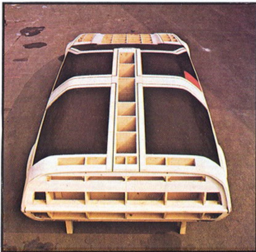
Early stages in the sketch-book life of the VW Porsche Tapino and also the wooden buck from which the skin was formed
