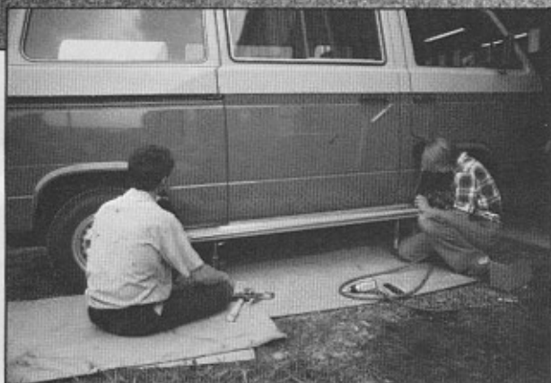
TOP, we couldn't think of a better application for a running board than on a new VW Vanagon. If you think we're wrong, take into account that a three-year-old kid can't step up like you can. BOTTOM LEFT, installation is fairly easy, but does require some tools and two hydraulic jacks. It's not a bad idea to have a friend help, too. BOTTOM RIGHT, "boards" are also available for the new VW pickup. Looks good with the Kamei flares and spoiler added.
