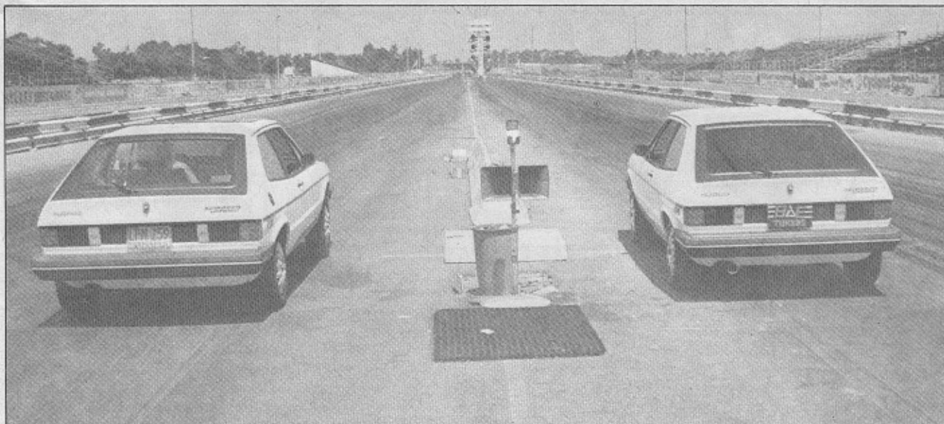
Head-to-head testing at OCIR proved the turbocharged Scirocco to be a full 2.4 seconds faster in the quarter mile! Note larger exhaust pipe on turboed car on right.
