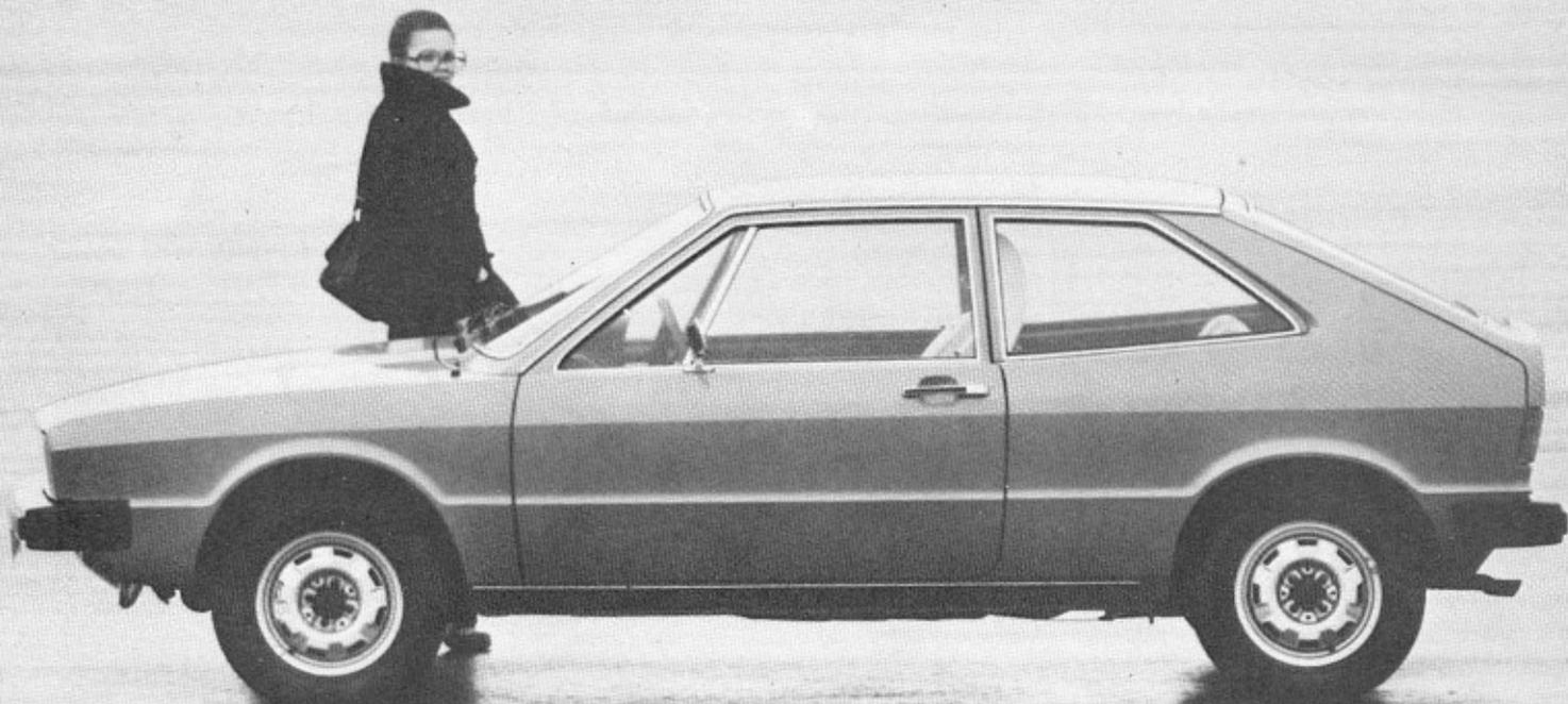
Compact dimensions and low roofline of the Scirocco are clearly evident in this view.
