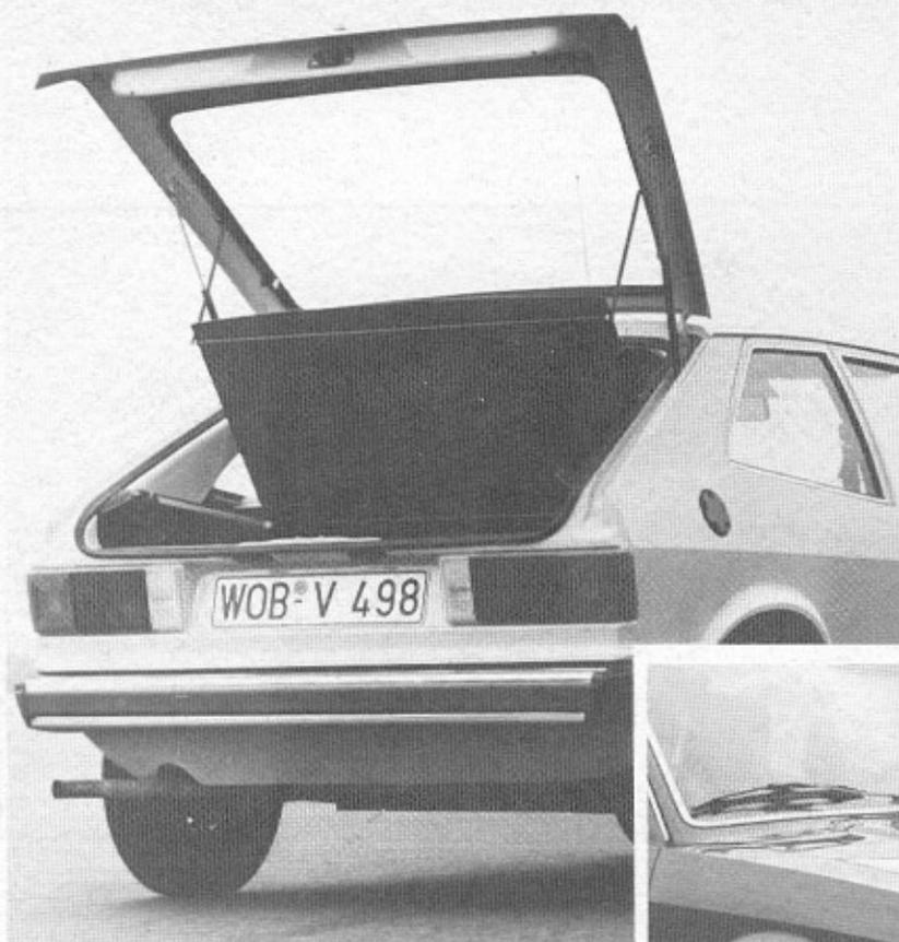
Scirocco features a lift-up third door which has fabric "shelf" attached to it to conceal luggage when door is in down position.
