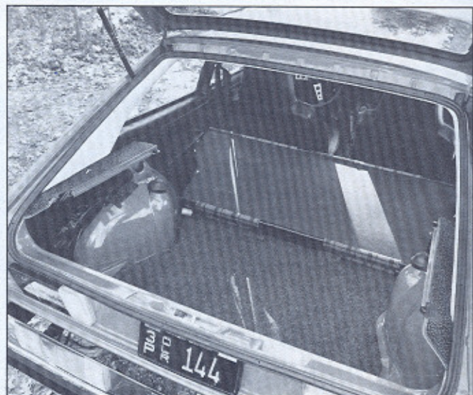
Scirocco's trunk is deep and spacious, but folding the rear seatback over doesn't produce a flat cargo floor. Divider panel comes out easily.
