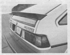
Scirocco's rear quarters is as large as the sheet metal will allow and all of it is recessed. But the most striking piece of all is the huge, curved back light. It is so large that the polyurethane spoiler is positioned over rather than underneath it. According to VW, this new air foiler cuts rearend lift by 60%, and it is attached to the car only at the ends. The resulting central slot al-
