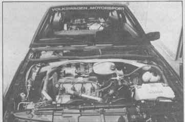
To get the axle line in the right place, the rear engine is located in what would be the load space of a normal Scirocco. The gear linkage running fore and aft can be clearly seen underneath the floor pan, as can the new, tubular, fabricated rear wishbones
