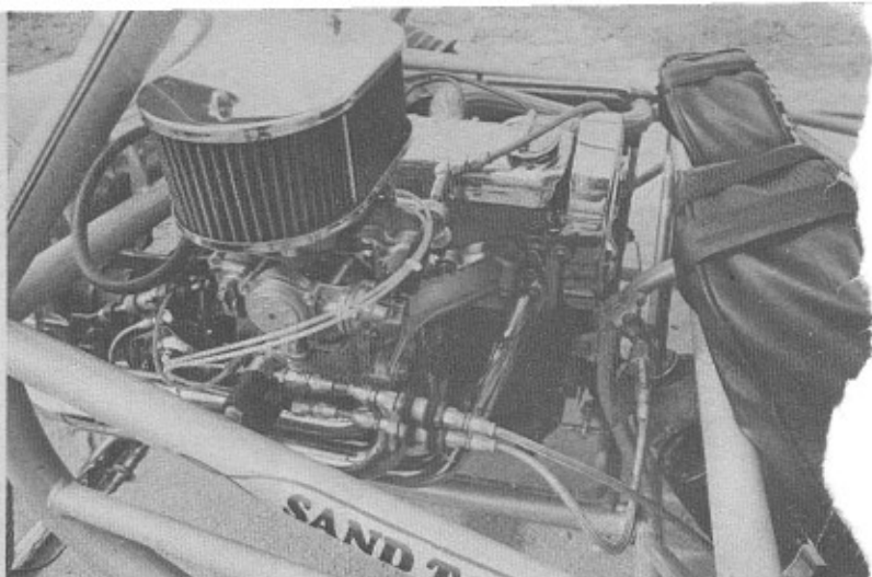
LEFT, the radiator is mounted at the side and uses an electric fan. RIGHT, engine is highly chromed and displaces 1600cc of overhead cam power. Nitrous Oxide system is used and a turbo is soon to come.
